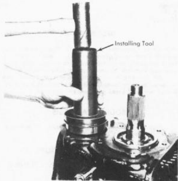
Fig. 18 Installing rear counter gear bearing
